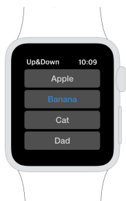
Figure 5: Our smartwatch application. It consists of total 26 words, each of which is as easy noun starting with a letter from A to Z. All words are arranged in a hierarchical order. The blue highlight acts as a cursor that the user can move around. The cursor goes up and down by turning PairRing.
