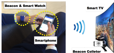
Figure 1: The research prototype system comprises a smart watch with a beacon, a smartphone, and a smart TV with a beacon collector.
