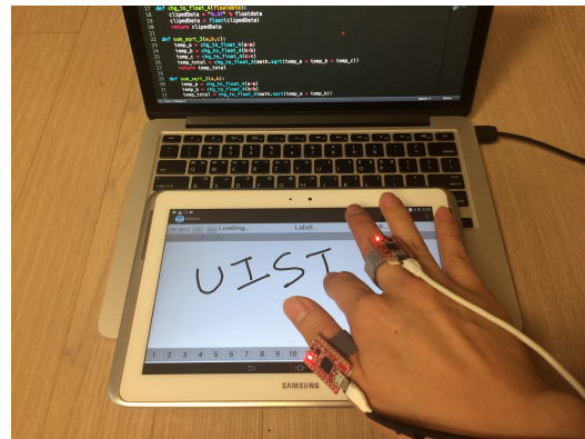
Figure 3. Our Touch+Finger prototype consisted of two ring-like devices with a IMU sensor attached, a touch-based device, and a PC for data processing
